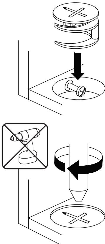
**EN\_Quickfit head** should be in the centre of the cam lock when the two panels are joined.
