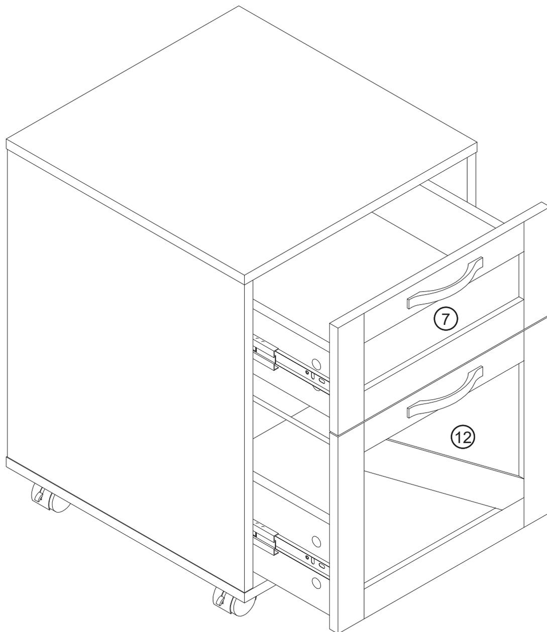
**EN** Be careful to push in the board when the both sides slide way been aligned.
