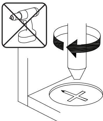
**EN**\_Turn cam lock clockwise to tighten.
