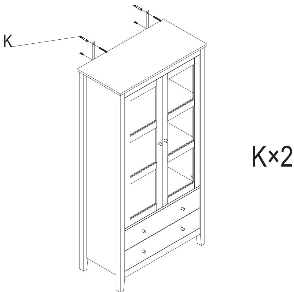
**EN** If it is a solid wall, please use expansion and self-tapping screws, if it is a wooden wall, only use self-tapping screws, please do not overtighten the screws
