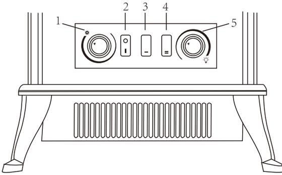
1. Thermostat control knob ( TEMPERATURE SETTING)- Adjust to maintain room temperature.
