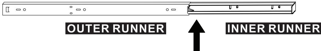
**EN\_Press and hold the drawer runner lock and then continue to slide drawer runners apart, as shown.**
