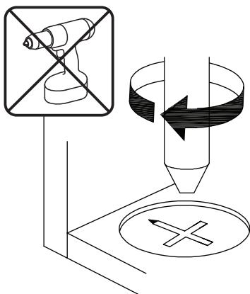
**EN**\_Turn cam lock clockwise to tighten.
