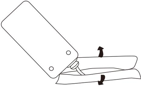
Tear off the bottom velcro and take out the battery.
