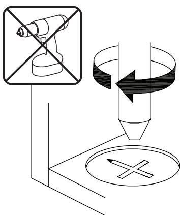
**EN** Turn cam lock clockwise to tighten.
