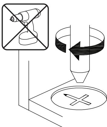
**EN**\_Turn cam lock clockwise to tighten.
