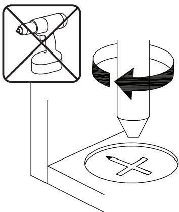
**EN**\_Turn cam lock clockwise to tighten.
