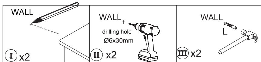
**EN** If it is a solid wall, please use expansion and self-tapping screws, if it is a wooden wall, only use self-tapping screws, please do not overtighten the screws
