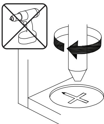
**EN**\_Turn cam lock clockwise to tighten.
