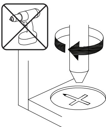
**EN**\_Turn cam lock clockwise to tighten.
