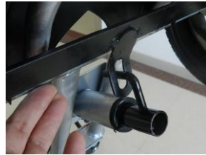
B. Make the steering shaft through the front frame
