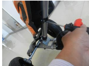
F. Fix the top of front panel
