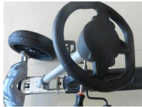
D. Fix the steering wheel on the steering shaft and fix it with screw 5*35
