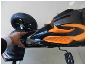
E. Fix the front pane on the frame and fix it with crew 4*10
