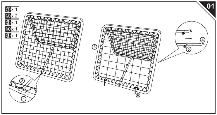
How to fold: Disassemble the screw set and fold the frame.
