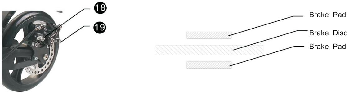
The brake pad and brake disc must be adjusted regularly as shown in the figure above. Leaving the brake pads and discs unadjusted for a long time will reduce the durability of the pads and become a safety hazard.
