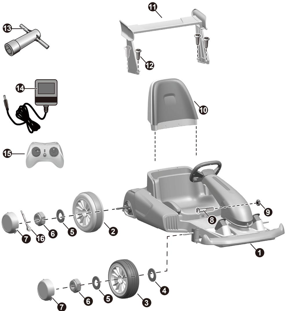
HINT: Some parts shown are assembled on both sides of vehicle
