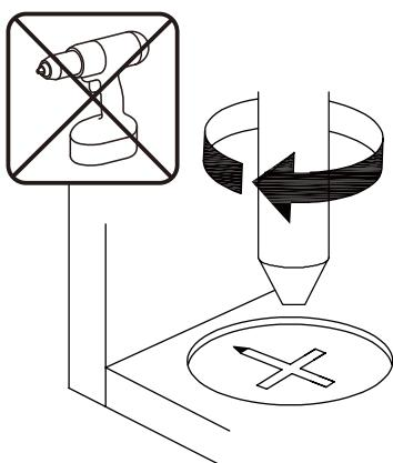
**EN** Turn cam lock clockwise to tighten.
