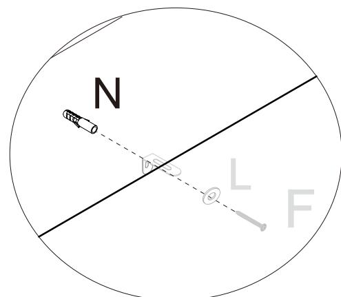
**EN** If it is a solid wall, please use expansion and self-tapping screws, if it is a wooden wall, only use self-tapping screws, please do not overtighten the screws
