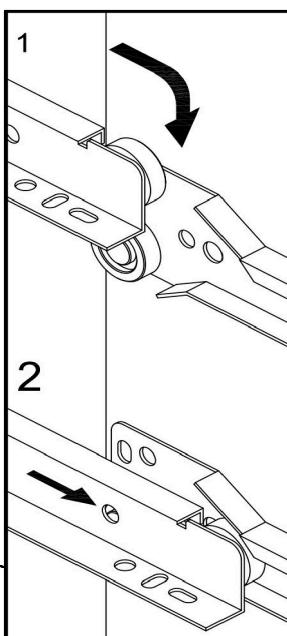
**EN** Be careful to push in the board when the both sides slide way been aligned.
