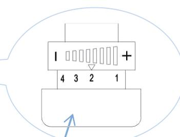
Note: Set the Tension Control Knob at 1 to ensure enough wire length to connect the Tension Control Wires (No. 72 and 73).
