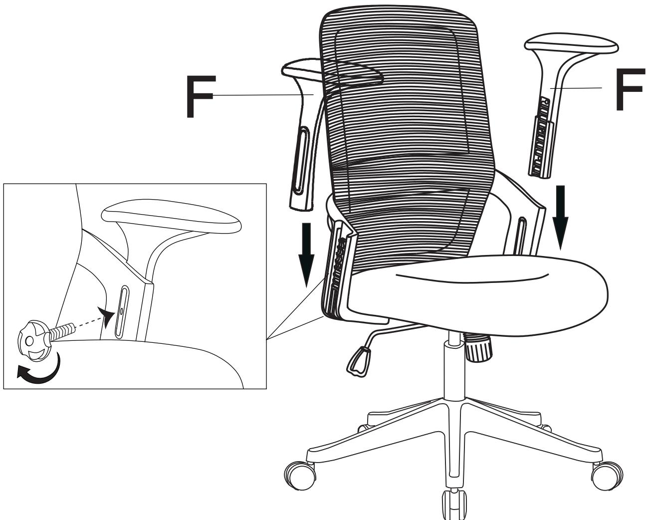
**EN** After the armrest is stuck, install and tighten it with the KNOB.
