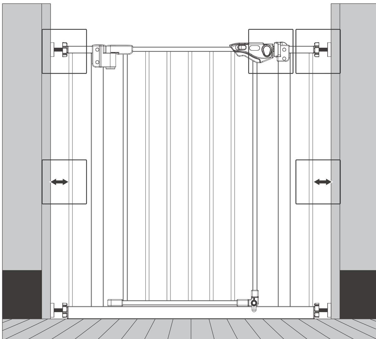
**NOTE** The gap between the gate and the wall should not exceed more than **2.5 inch** on either side (*Figure 3-4 and 3-5*)
