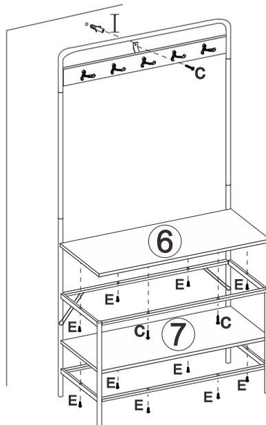
**EN** If it is a solid wall, please use expansion and self-tapping screws, if it is a wooden wall, only use self-tapping screws, please do not overtighten the screws
