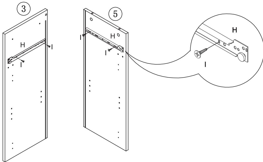
**EN** Please find the exact hole for installation, otherwise it will be misaligned. The screws on the drawer slide must be leveled , otherwise it will affect the smoothness of the d rawer.
