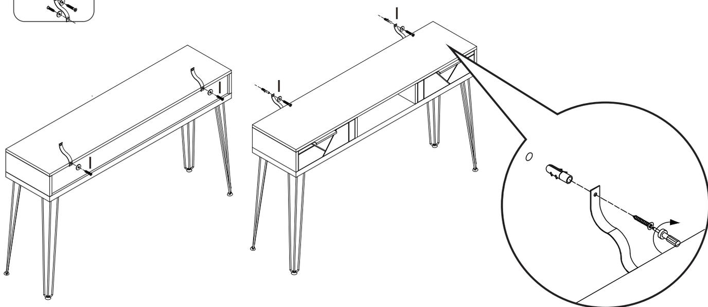
**EN** If it is a solid wall, please use expansion and self-tapping screws, if it is a wooden wall, only use self-tapping screws, please do not overtighten the screws
