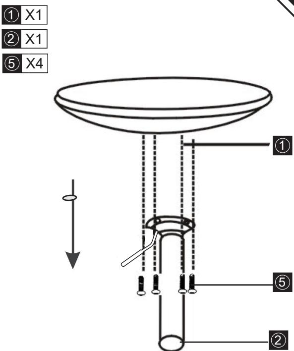
**EN:** The round hole on the table surface and the handle are the same direction.
