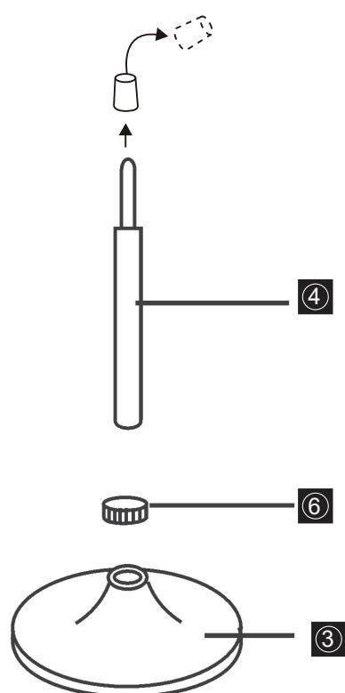
**EN:** The hydraulic cylinder has a cap on the top of it that must be removed prior to assembly.
