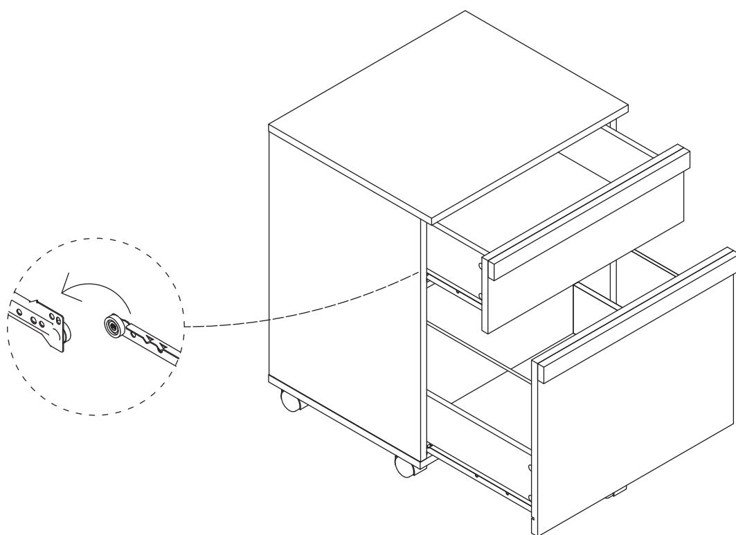
**EN** Be careful to push in the board when the both sides slide way been aligned.
