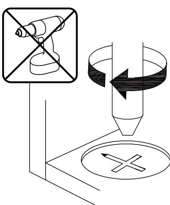
**EN** Turn cam lock clockwise to tighten.
