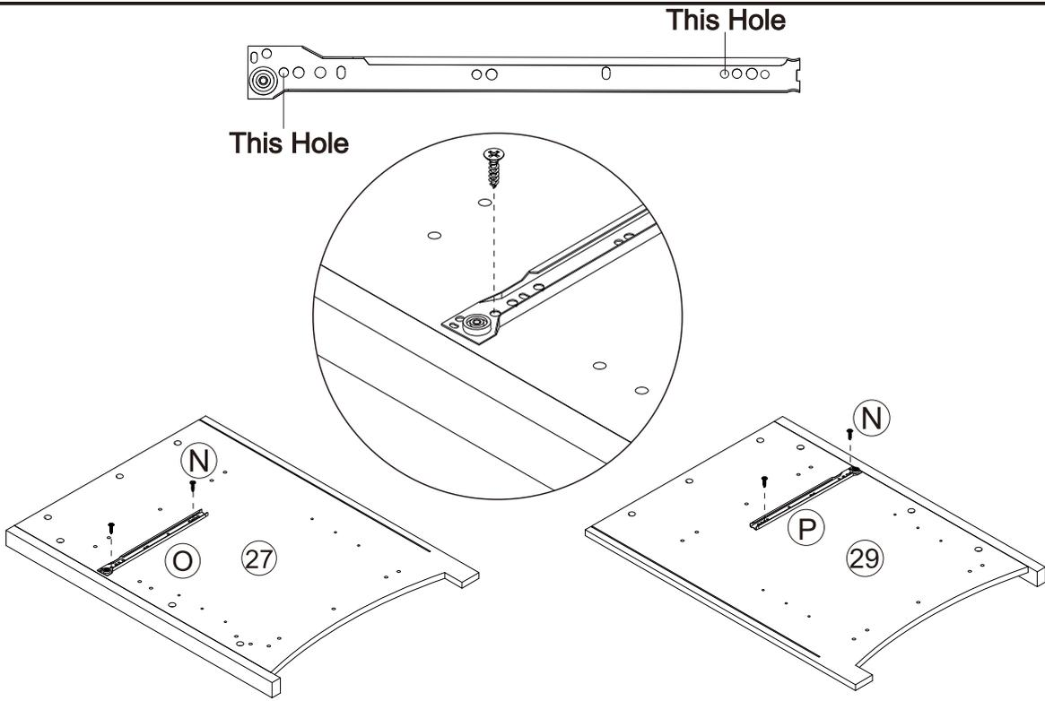
**EN\_**Please find the exact hole for installation, otherwise it will be misaligned. The screws on the drawer slide must be leveled, otherwise it will affect the smoothness of the drawer.
