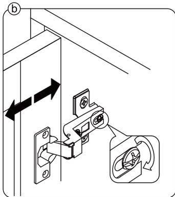
**EN** To adjust the gap from the door to the main frame turn the screw clockwise or anti-clockwise as needed.
