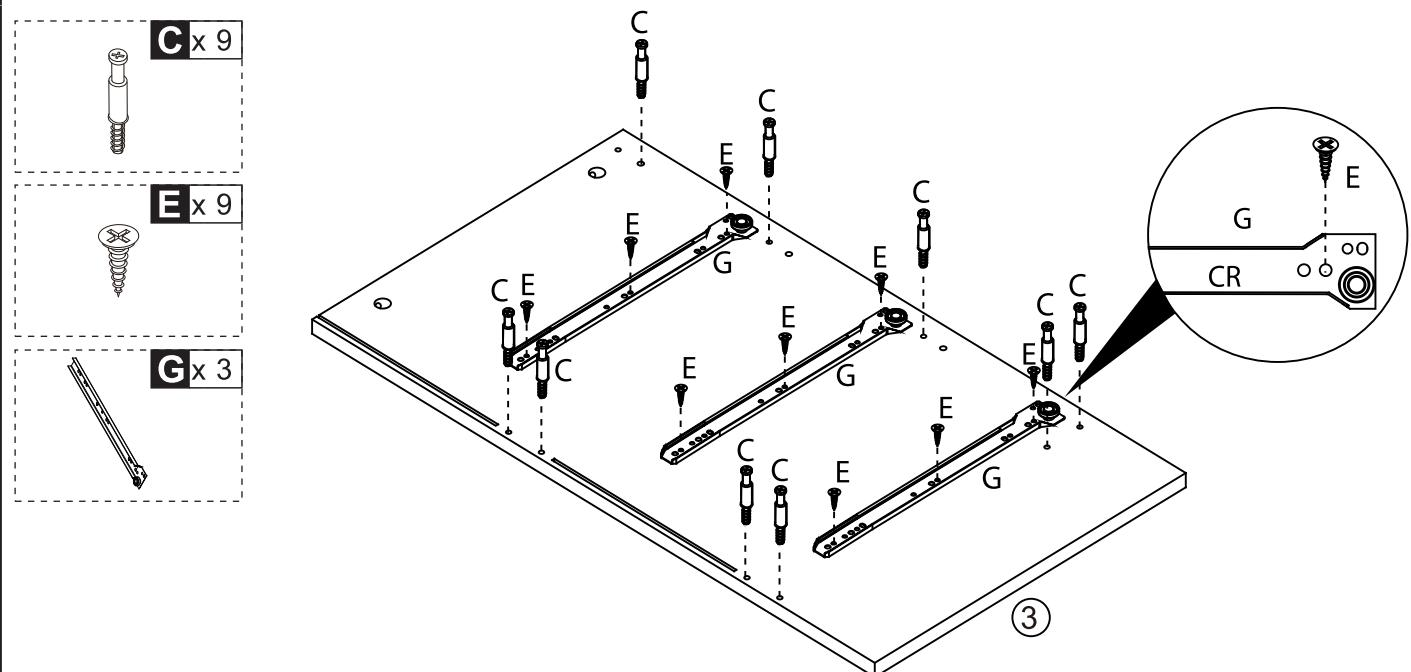
**EN** Please find the exact hole for installation, otherwise it will be misaligned. The screws on the drawer slide must be leveled , otherwise it will affect the smoothness of the d rawer.
