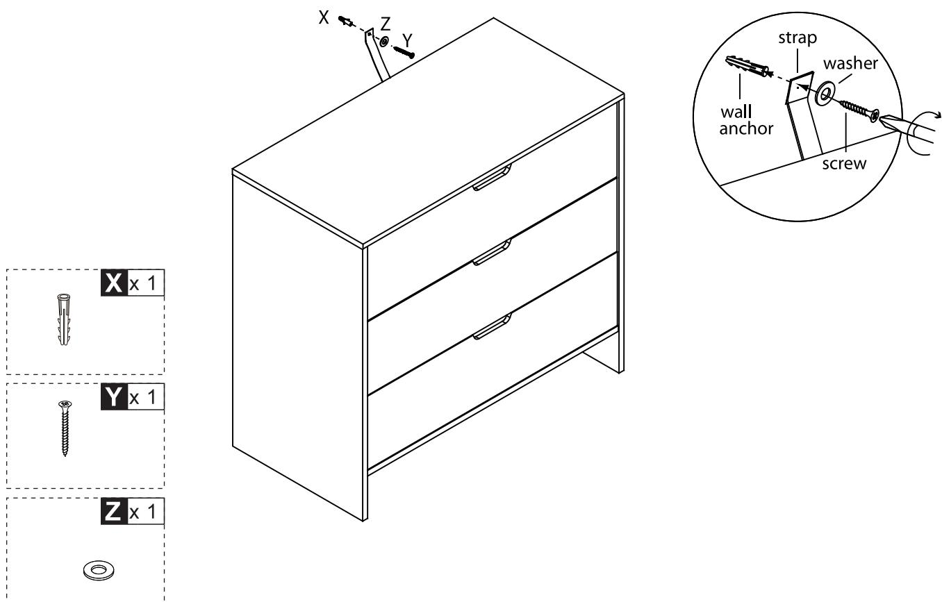
**EN** If it is a solid wall, please use expansion and self-tapping screws, if it is a wooden wall, only use self-tapping screws, please do not overtighten the screws
