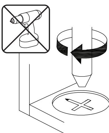
**EN**\_Turn cam lock clockwise to tighten.
