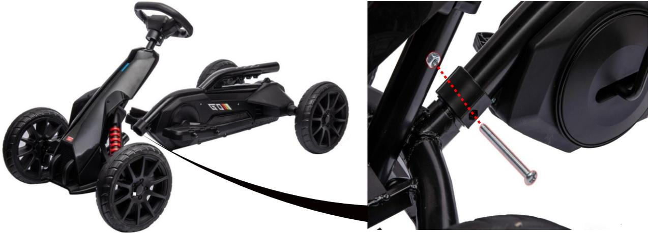
Connect the front assembly to main body as picture shown and fasten fix it with nut and screw.
