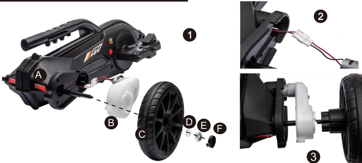
A. Main body    B. Gear box    C. Wheel    D. Washer    E. Nut    F. Wheel cover
