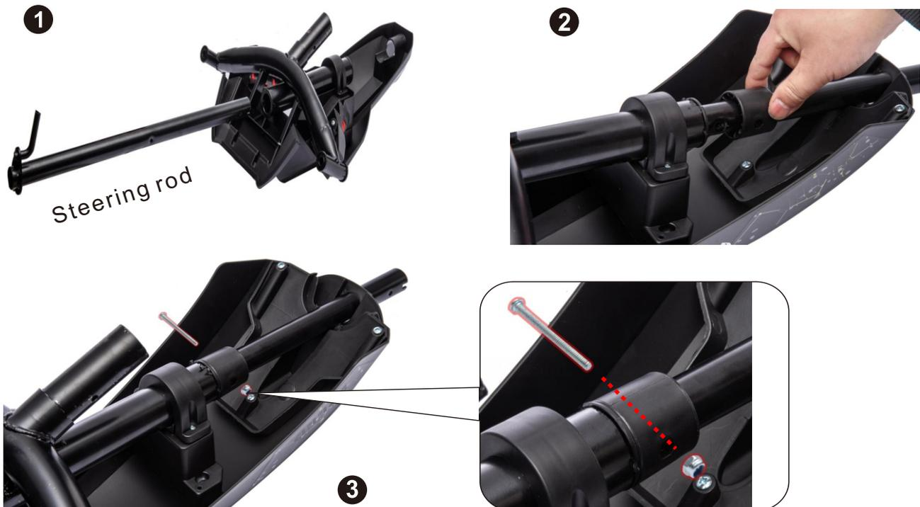
1. Insert the steering rod under the front assembly as picture shown.
