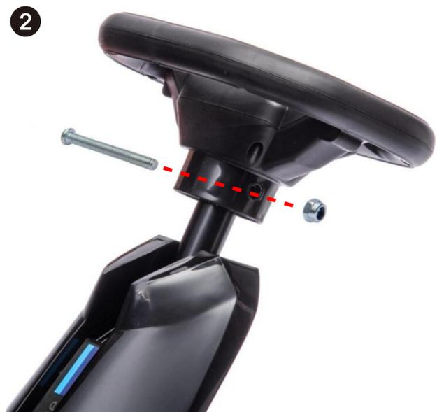
1. Put steering wheel to the rod as picture shown, make sure all holes in one line.
