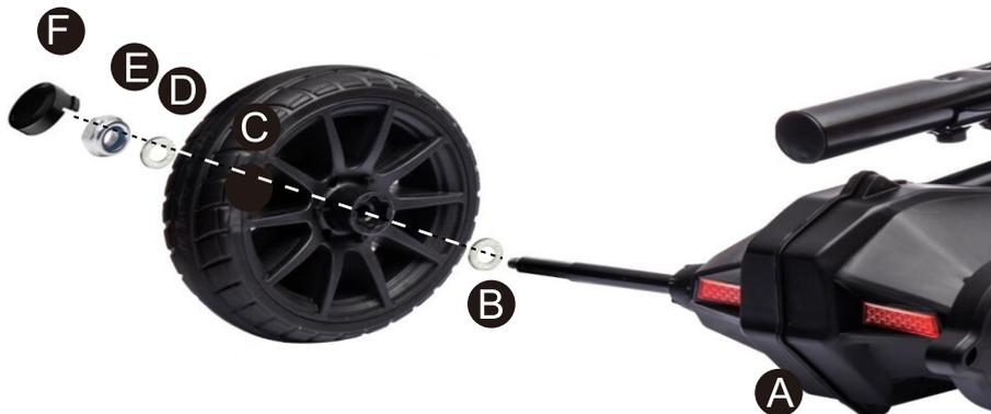
A. Main body    B. Washer    C. Wheel    D. Washer    E. Nut    F. Wheel cover
