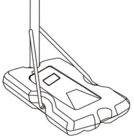
Fix the other end of Pole Brace(L1)&(L2) on two sides of Base(S) by Bolt Set (C1), (C2)&(C3) as shown.
