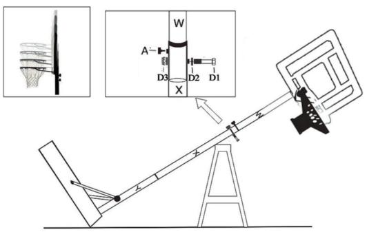
Insert the Top Pole(W) into Middle Pole (X), adjust it to required height, then fix them by Palstic Head Knob(A)&Bolt Set (D1), (D2)&(D3) as shown. Adjust the height by change the Bolt Set (D1), (D2)&(D3) in different holes on Top Pole(W).
