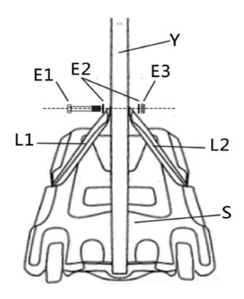
Fix one end of Pole Brace(L1)&(L2) on Bottom Pole(Y) by Bolt Set (E1),(E2)&(E3) as shown.
