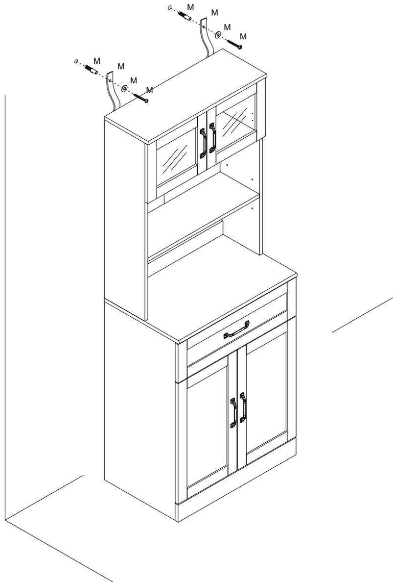
**EN\_ If it is a solid wall, please use expansion and self-tapping screws, if it is a wooden wall, only use self-tapping screws, please do not overtighten the screws**
