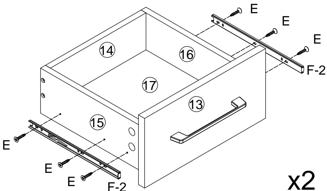
**EN** Please find the exact hole for installation, otherwise it will be misaligned. The screws on the drawer slide must be leveled , otherwise it will affect the smoothness of the d rawer.
