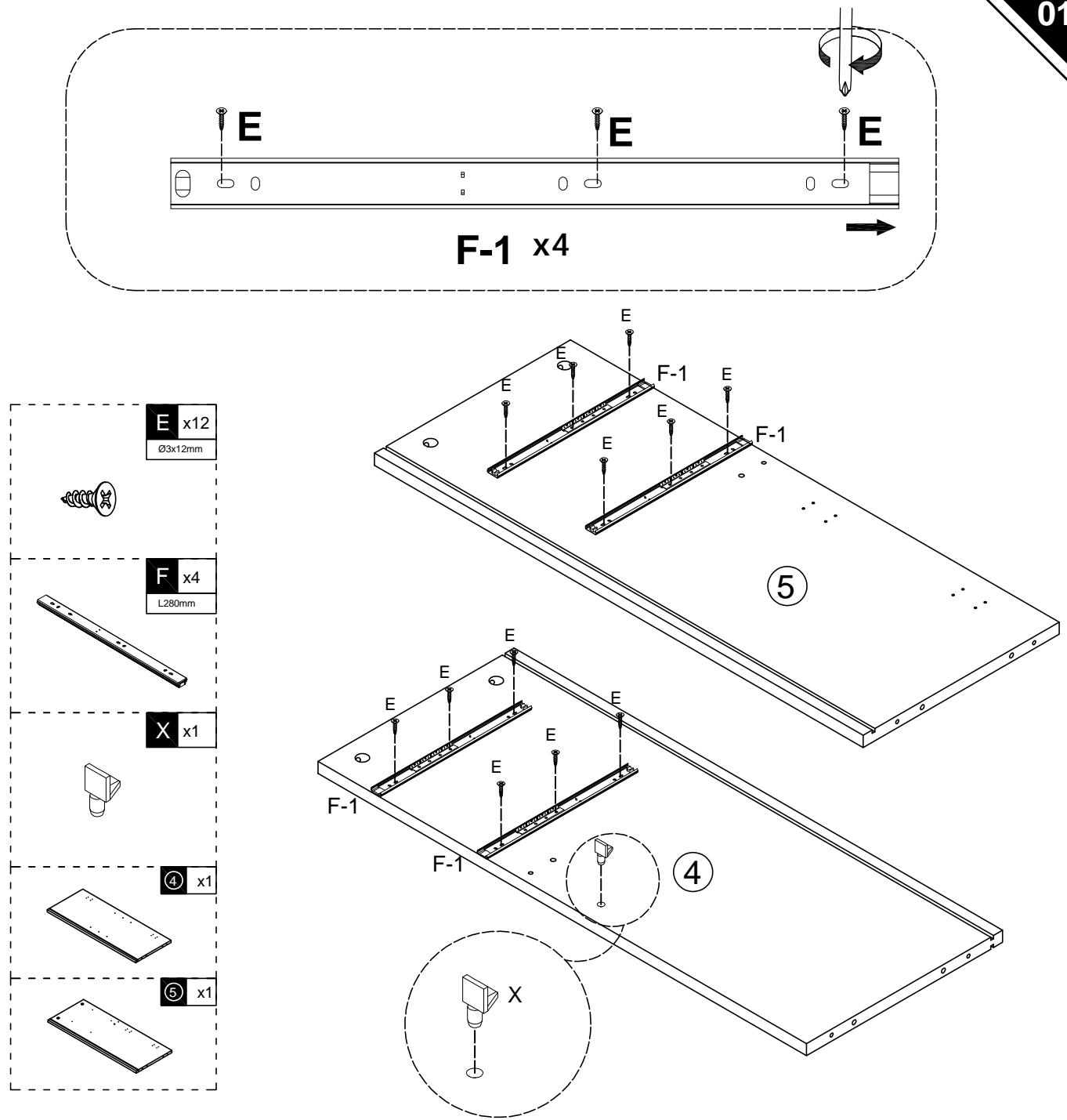
**EN** Please find the exact hole for installation, otherwise it will be misaligned. The screws on the drawer slide must be leveled , otherwise it will affect the smoothness of the d rawer.
