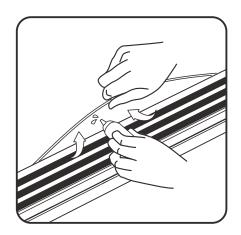
3. Adjust tightness of running belt. All treadmills shall be adjusted for tightness before delivery and after installation. However, the running belt may be loosened after a period of use.
