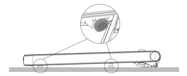
3.To move the walking machine: You must unplug the power first, then lift the tail of the walking machine by hand, and the front moving wheel touches the ground to move the walking machine back and forth.
