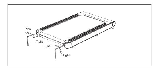
Please adjust the right bolt clockwise or left bolt counterclockwise if the running belt is right deviation.
