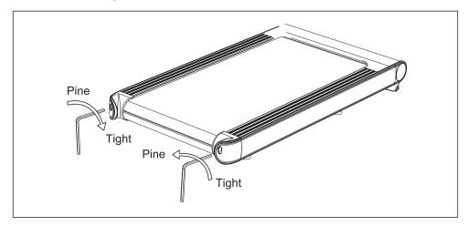
Please adjust the left bolt clockwise or right bolt counterclockwise if the running belt is left deviation.
