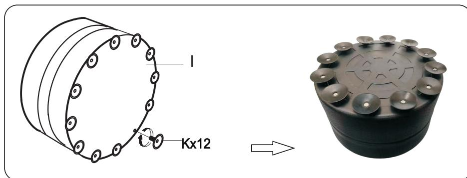
3. Turn the base upside down, theseis a sand injection hole with a diameter of 3 cm at the bottom, add sand and water to two thirds of the sand bag, and close the lid.
