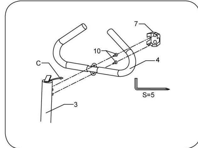
Pull Connector C through the meter holder of the upper tube. Fix and fasten the handle to the upper tube with a bolt and then put on the cover, as shown on the left.
