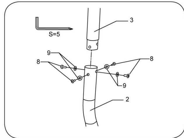
Pull Cable B through the upper tube, which is then fastened to the lower tube with a bolt, as shown on the left.
