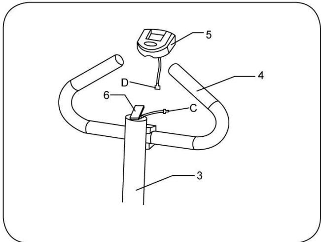
Connect Connector C and meter plug D, and then fix the meter on the meter holder.
