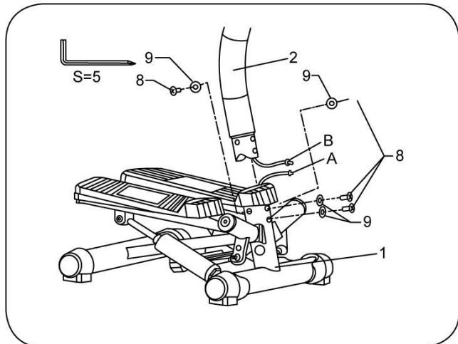
Place the base machine on a flat surface. Insert Cable B into the lower tube, and connect Cable A and B together, and then insert the lower tube into the base machine and fasten with a bolt, as shown on the left.
