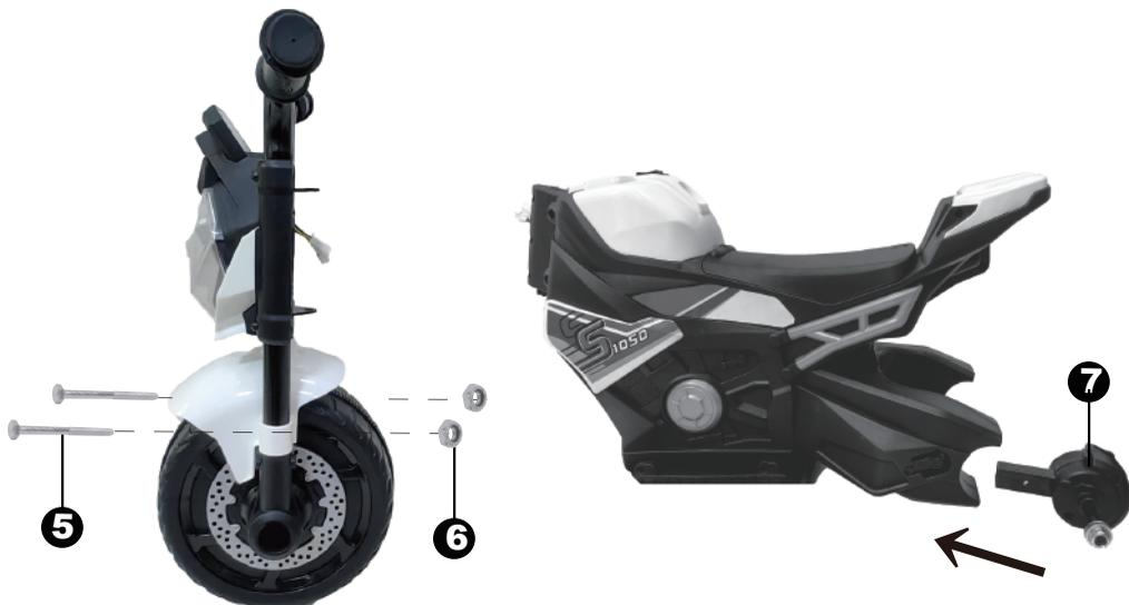
**D****Install rear wheels and handlebars**
