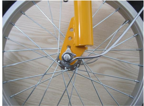
5: The front wheel axle is stuck in the front fork groove, then insert the safety hook.
