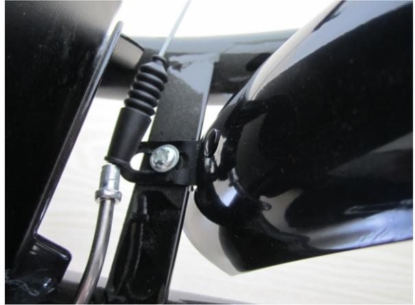
1. The fixing piece of the rear fender is installed in the hole of the frame, tighten the screw.
