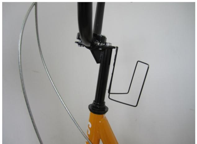
Loosen the nut, insert the bottle cage, and tighten it firmly.
