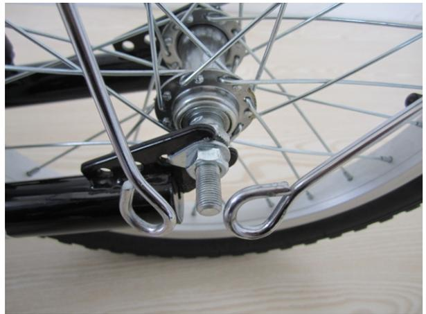
2. The rear wheel axle is stuck into the rear fork groove, then insert the safety hook.
