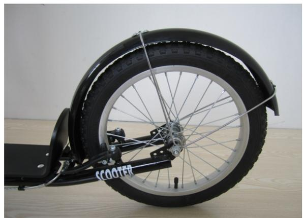
4. Set the fender support into the rear axle and tighten the outer nut to fix the fender support.
