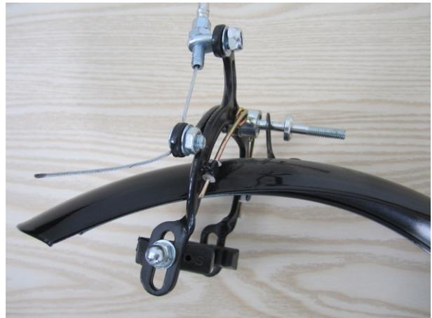
1. The front fender fixing piece is inserted into the front brake screw.
