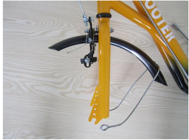
3: Insert the front brake screw into the hole of the front fork riser.
