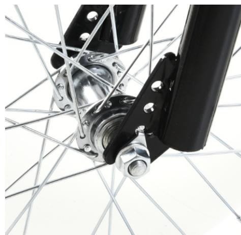
Please do not unscrew the two sides of nuts (c). The clearance between the bearings was adjusted at the factory.
