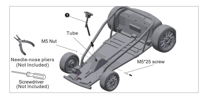
② Thread the steering axle **6** through the car body and steering wheel rod from the bottom. Insert the hook on the steering wheel axle **6** into the hole on the front axle, as shown in picture (a). Ensure the top part of the steering axle **6** extends beyond the steering wheel rod.
