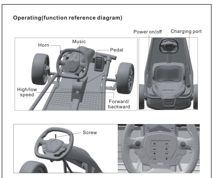
Before first use, insert four AA 1.5V alkaline batteries. Note: The steering wheel has a horn and music function.
