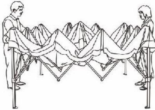
**EN\_3.** Each person should then grasp the bottom of the middle frame section (cross beams) where it forms diamond. Lift slightly and slowly walk backward until the frame is fully extended. Be careful not to pinch your finger or pull backward too hard as this may result in the bending of cross beams.
