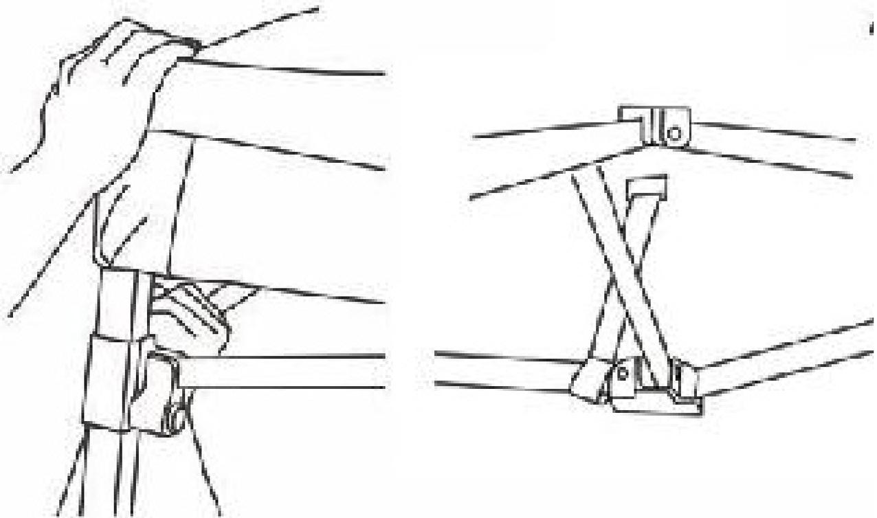
**EN\_4.** Engage the slider at each corner by pushing up the slider with one hand while holding down the top of the leg with the other hand. Repeat this at the rest of corners.
