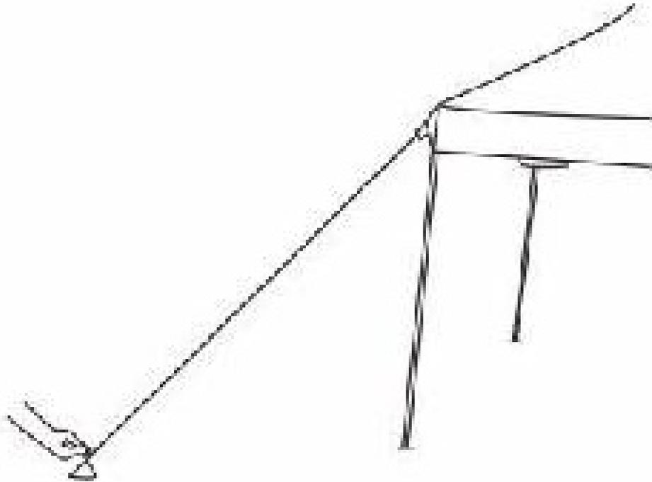
**EN\_7.** Measure out from the leg to a proper distance and secure the four anchors to ground at a 45 degree angle. Tie up one end of each guy(D)rope to the triangular shaped rope holder located on the outside fabric corners. Tie the other end of each rope to the anchor on the ground. Make sure the guy ropes have the proper tension.
