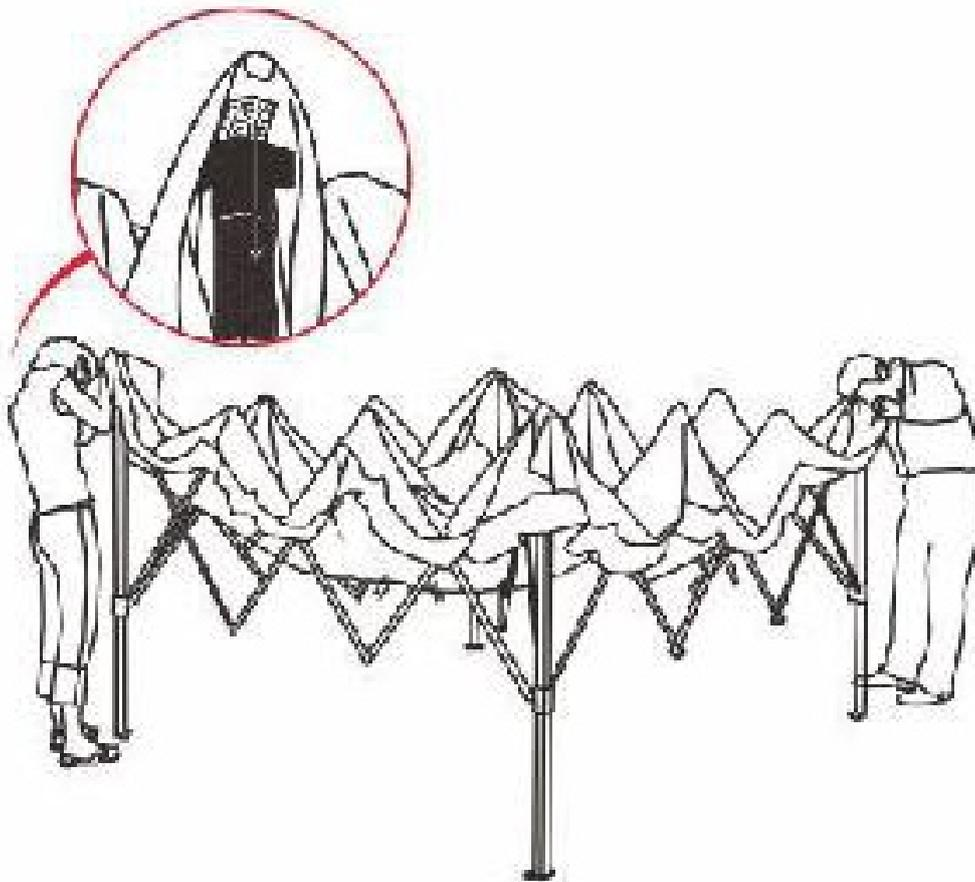
**EN\_2.** Place the Main Canopy (B) over the top frame. Use the Velcro pads to secure each corner of the canopy to the frame under the plastic leg caps.
