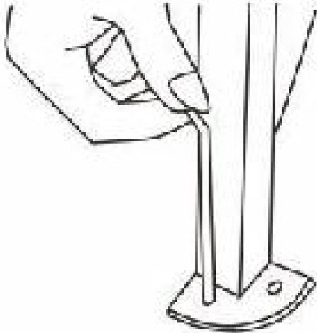
**EN\_6.** Stake (C) down the gazebo by driving the 8 anchors through one of the holes on each base foot. This will keep the leg from moving sideways in mild weather conditions.
