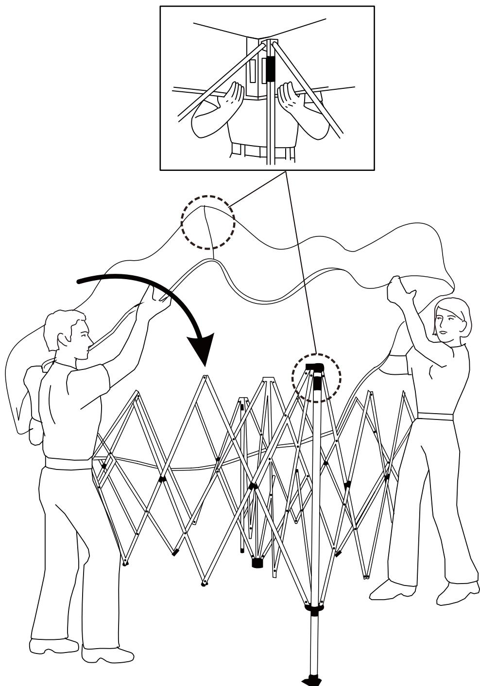
**EN** Place the canopy fabric on the frame and align the four corners of the canopy fabric with the four corners of the frame.
