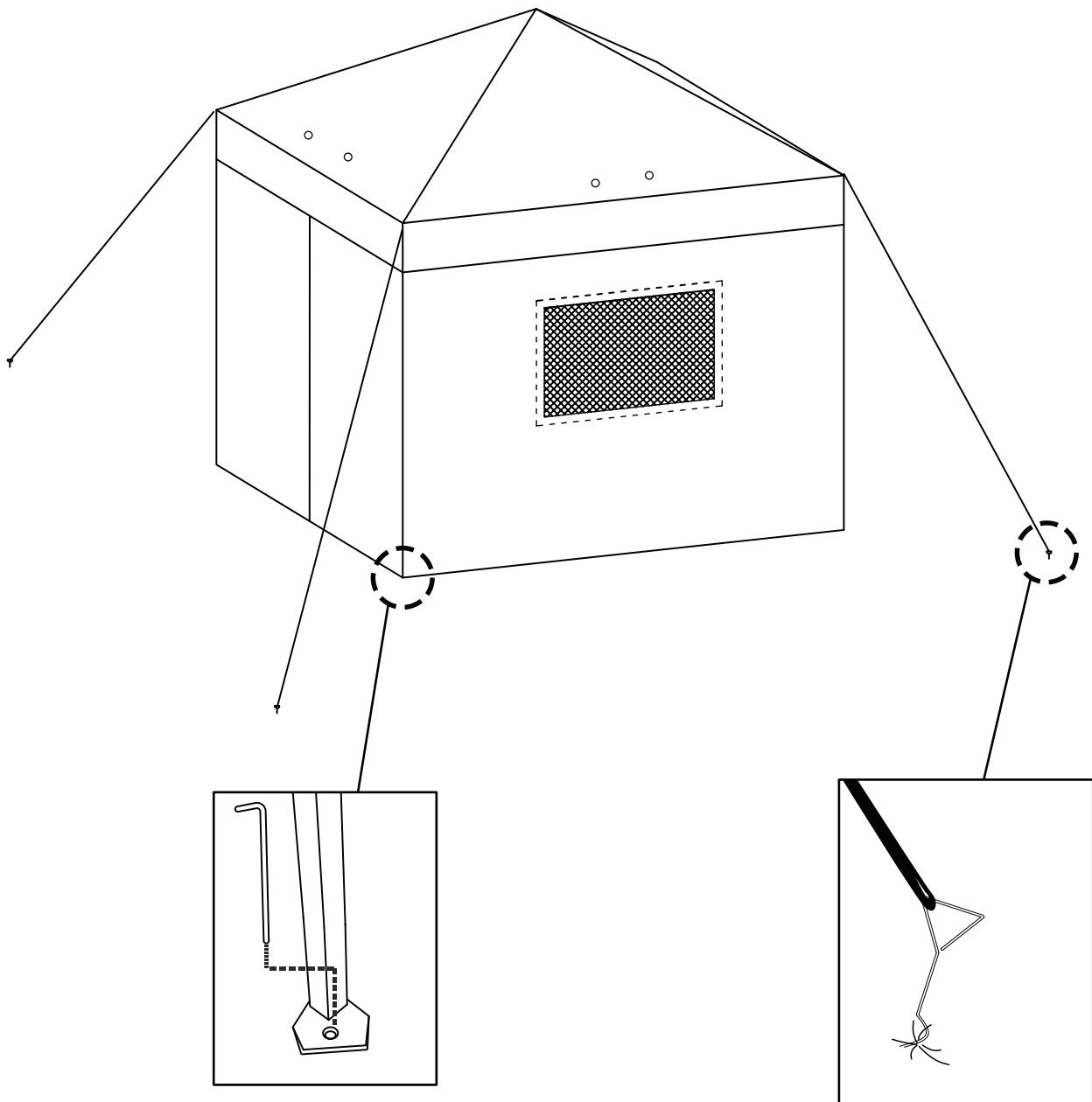
**EN** Connect the canopy fabric and the ground anchors with ropes, and fix the anchors into the ground for added stability.
