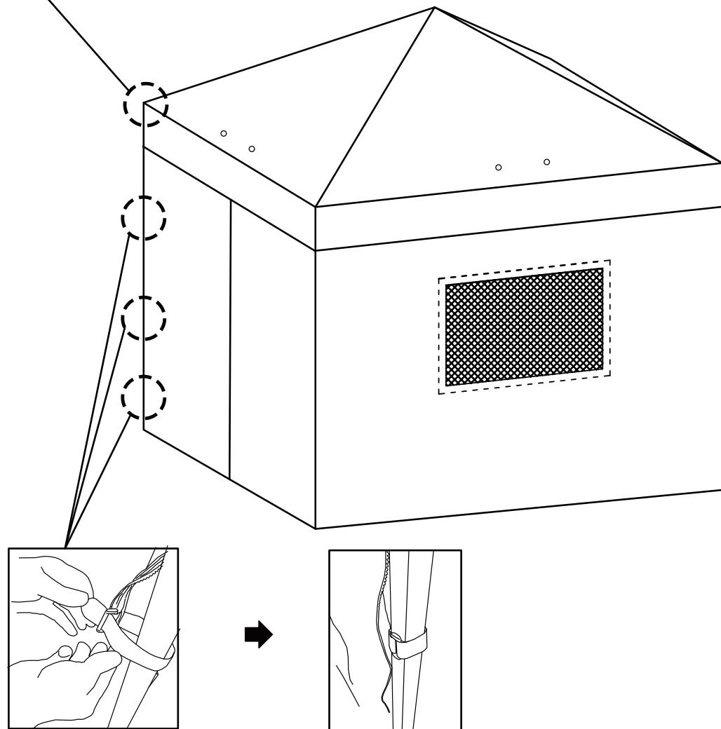
**EN** When assembling, please completely attach the of the wall as well as the door to the canopy fabric of the top before zipping the walls down.
