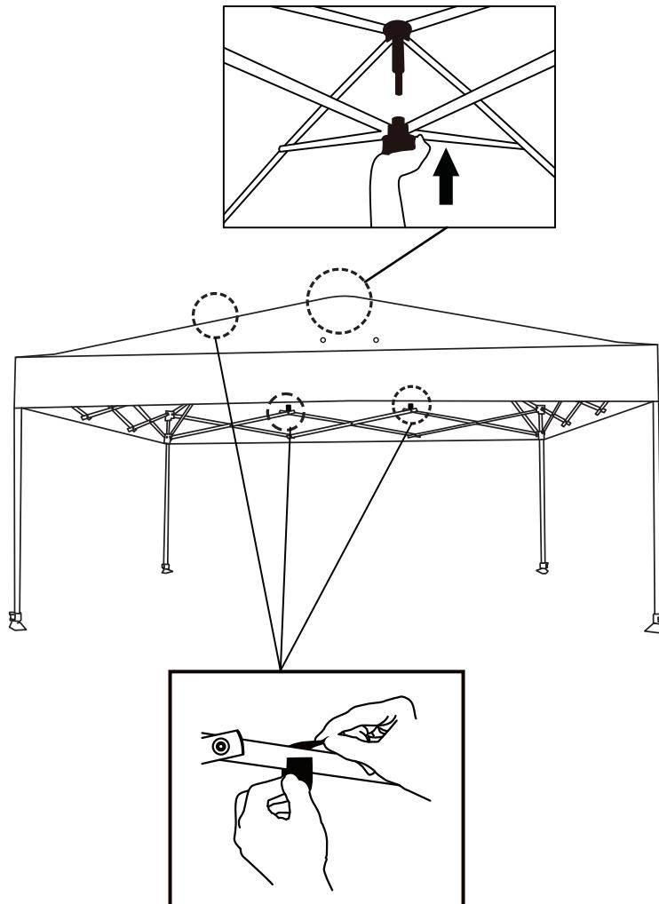
**EN** Attach the canopy fabric to the frame with the loop fasteners. Push up the central locking system until it locks into place and the entire frame is fully extended. After setting up the canopy fabric. Please reinforce the fabric to the frame with the loop fasteners inside the canopy.
