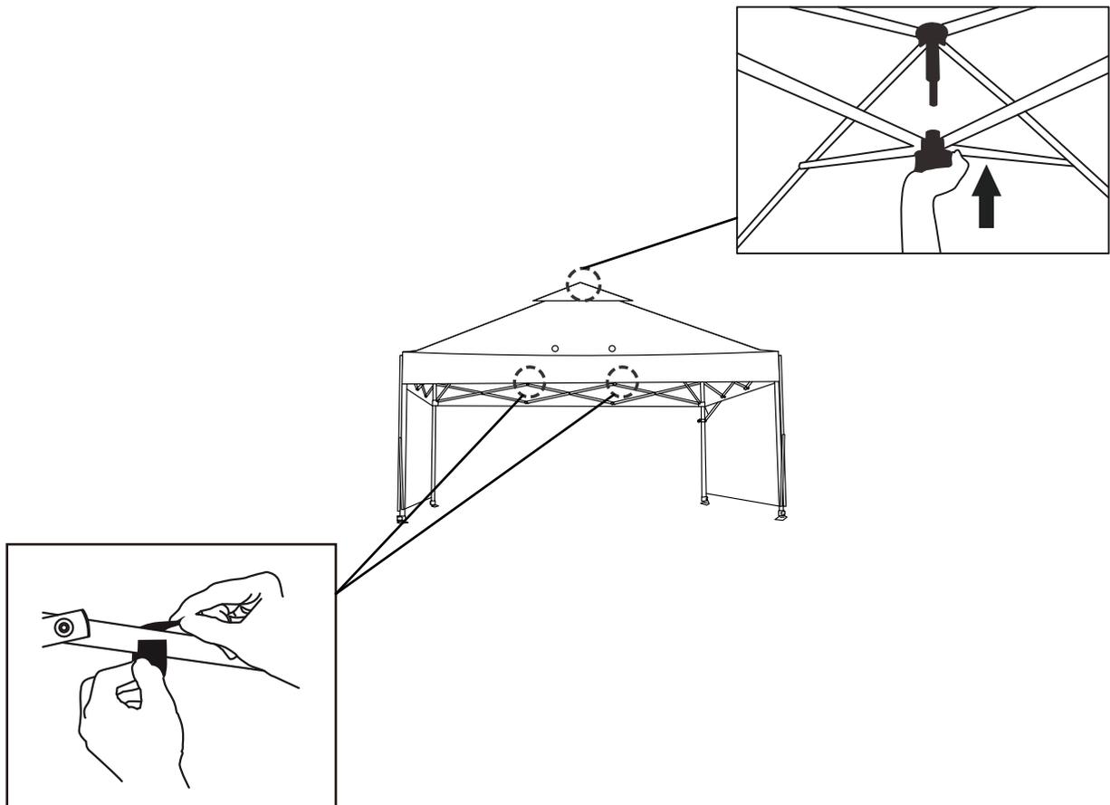
**EN** Attach the canopy fabric to the frame with the loop fasteners. Push up the central locking system until it locks into place and the entire frame is fully extended. After setting up the canopy fabric. Please reinforce the fabric to the frame with the loop fasteners inside the canopy.
