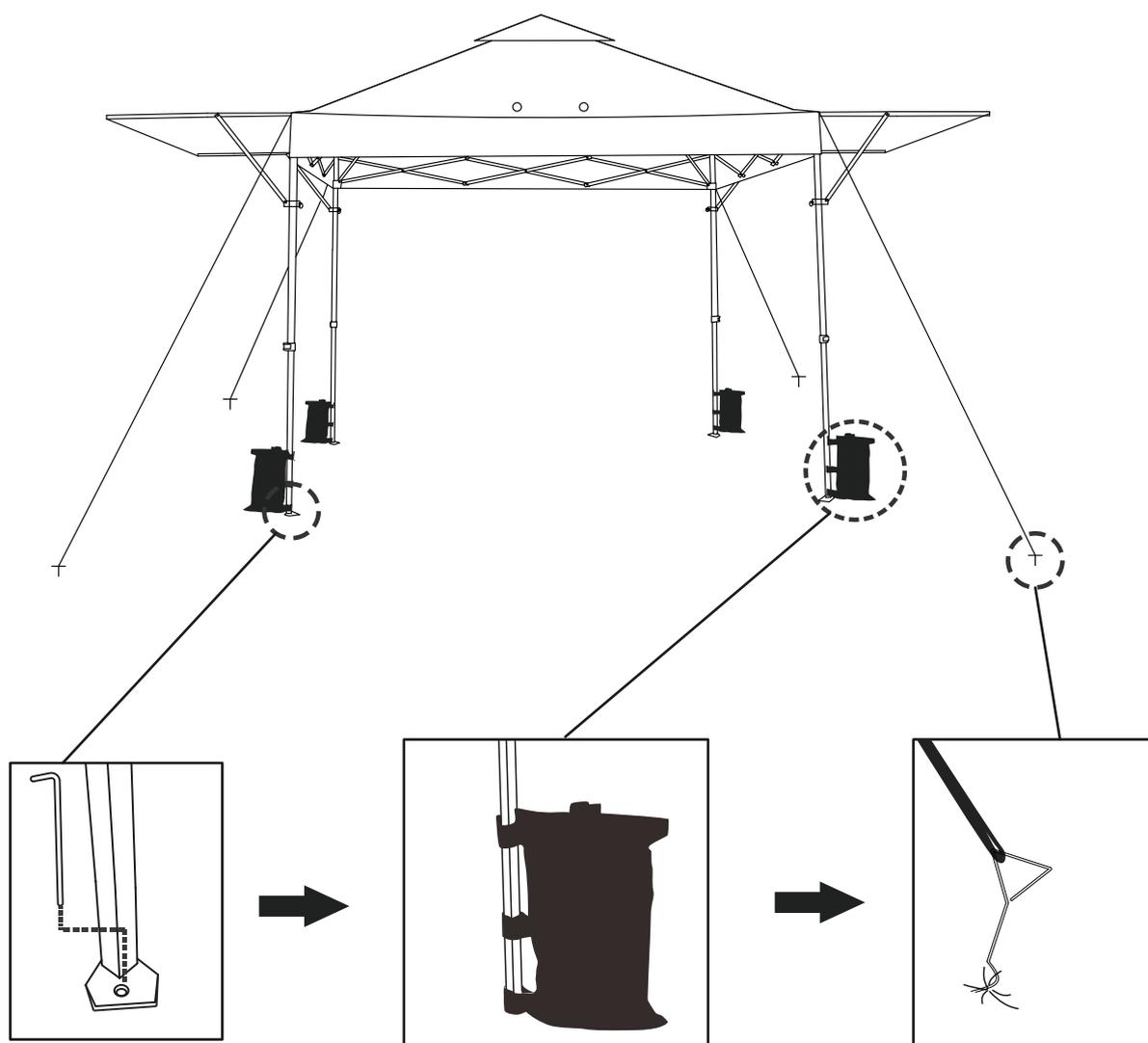
**EN\_** Fill up the sand bags and tie them to the frame legs. Connect the canopy fabric and the ground anchors with ropes, and fix the anchors into the ground for added stability.
