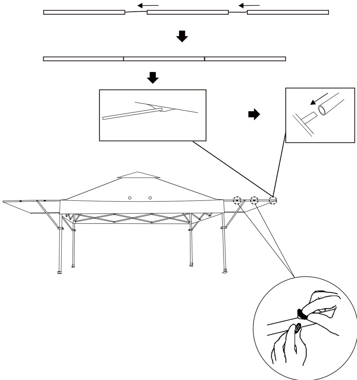
**EN\_** Install 3 circular pipes. First insert the circular tube into the side fabric, and then insert the circular tube into the small circular tube on both sides of the bracket. 2 holes on each leg for 2 adjustable heights. Adjust the side height by pulling the button and sliding the side tube along the legs. Extend Side tube to your desired height and the button will automatically lock in place. Please do not overextend the frame legs, otherwise the canopy fabric may be damaged.
