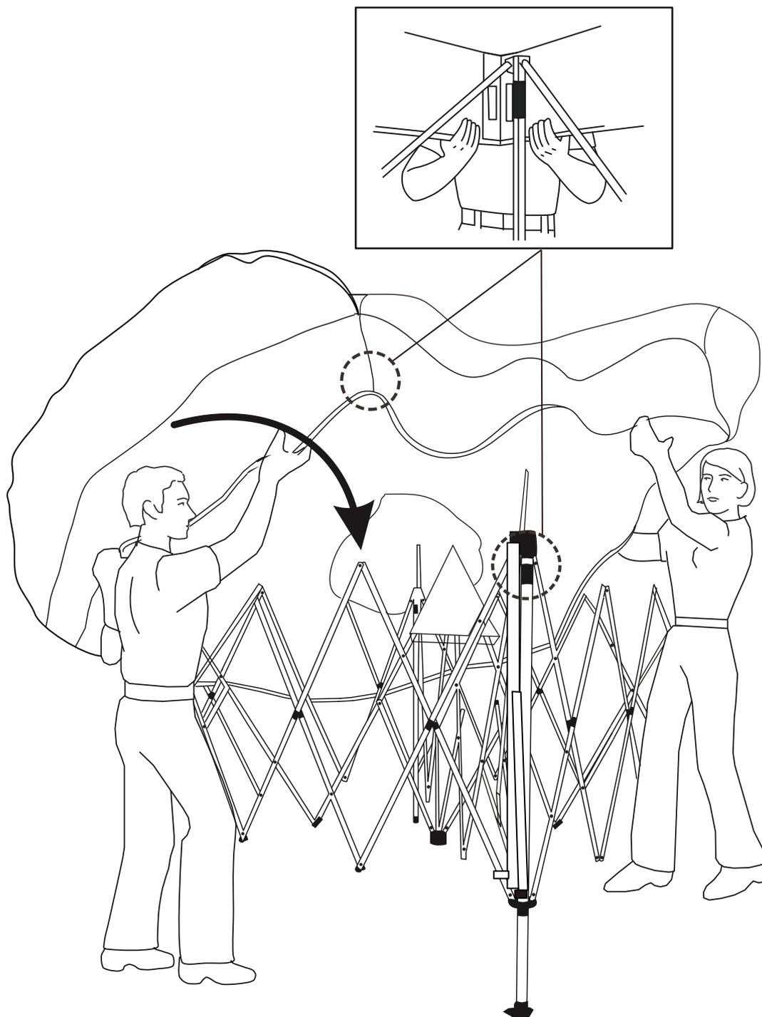
**EN** Place the canopy fabric on the frame and align the four corners of the canopy fabric with the four corners of the frame.
