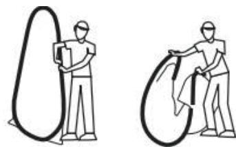
With a firm hold of all 8 bunched together poles, lift the tent and place one end on the ground - there should be a circle shape on the ground and another in front of you.
