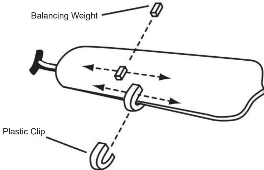
Note: prior to using this equipment check your fan to ensure it is correctly installed and all the blade adjustment screws are fully tightened.
