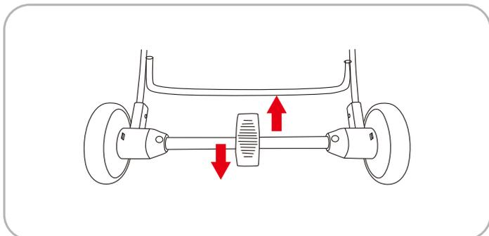
5. Press the middle brake lever to drive. Hook the middle brake lever.
