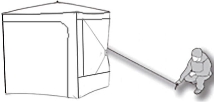
Find the side of the Fish Inn that faces into the wind and attach one of the provided straps to the center hubs of that wall. Stretch the strap into the wind and with the remaining Ice Spike(s), secure the strap to the ice.
