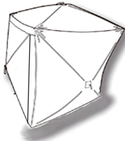
Lifting the roof of shelter up, pull outward on the center hub of one of the walls. Continue around the entire shelter,pulling each wall hub until all of walls are set up.
