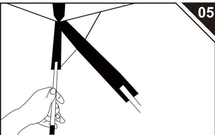
The external fiberglass rod was opened and placed in the ribbon inside the door and tied with a cloth in the middle. The corn holes at the four corners of the inner bottom are fixed with nails.
