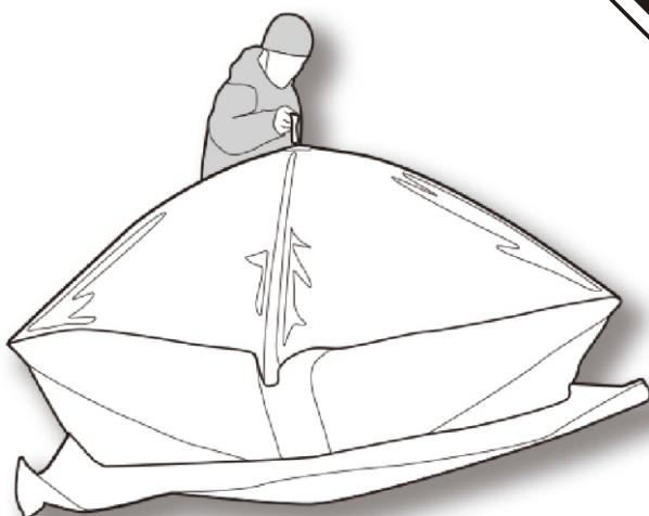
Firmly pull up on the strap in the center hub of the roof until it pops up. Twist the roof slightly so corners of top and bottom line up.
