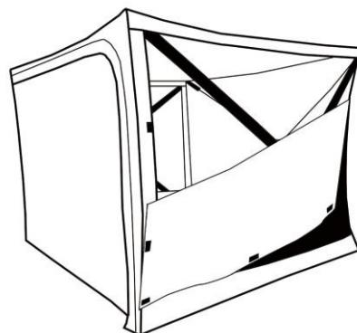
Paste the surrounding cloth on both sides of the tent according to the corresponding adhesive positions. Provide rain protection for the tent
