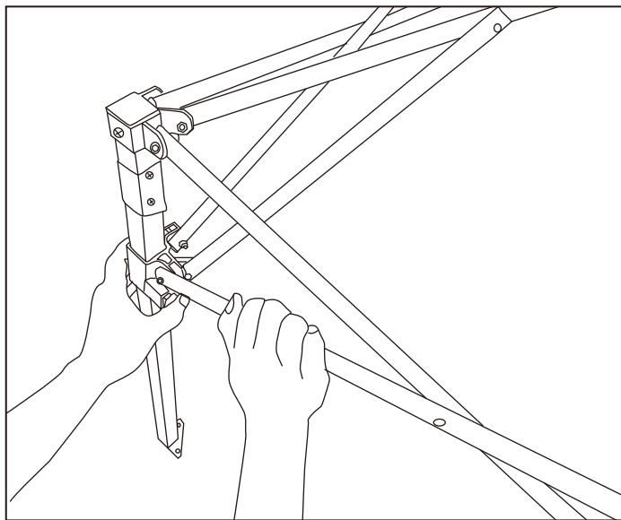
**EN** Release sliders at all four corners by pushing the red plastic button and gently push the sliders down to leave the locking position.
