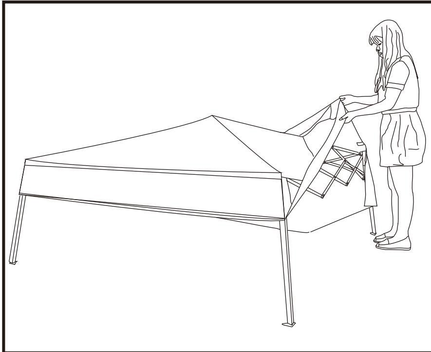
**EN** Remove the canopy top from the frame and fold it up nicely. Do not put it in the backpack before frame.
