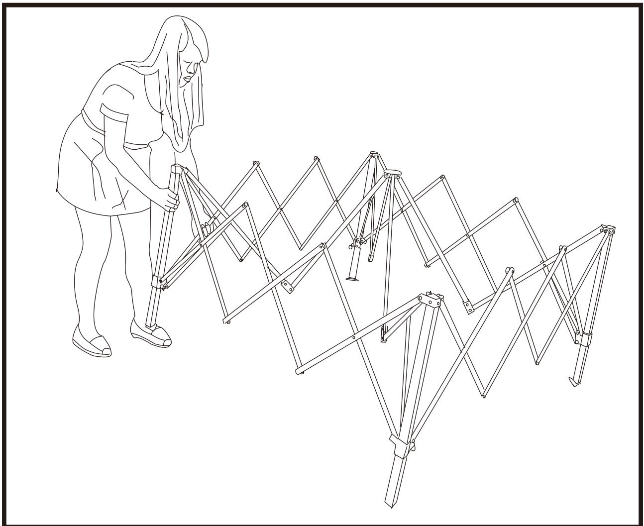
**EN** With all four pull-pin lock released , lift and walk one corner of the frame towards the opposite|corner to close the frame.
