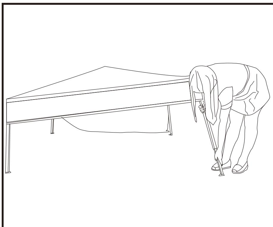
**EN**\_Release the spring button lock and shorten the telescoping legs.
