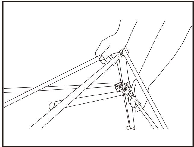
**EN** Engage the slider at each corner by pushing up the slider with one hand while holding down the top of the leg with the other hand until it locks in to place.
