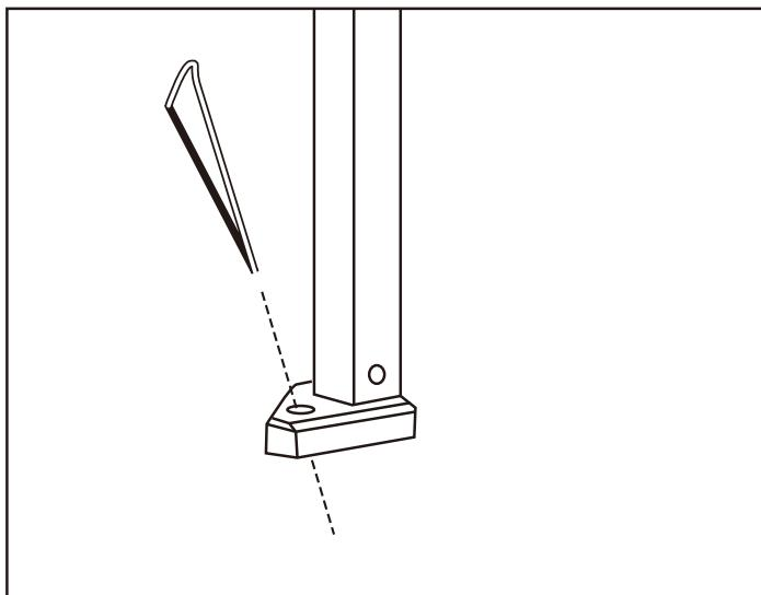
**EN** To assemble on a beach or in soft soil, use weights (sand bags or other heavy objects) on each foot or place legs twelve inches down into the sand or soil to help secure the set-up for beach use. Stakes alone will not secure the gazebo in sand or soft soil.
