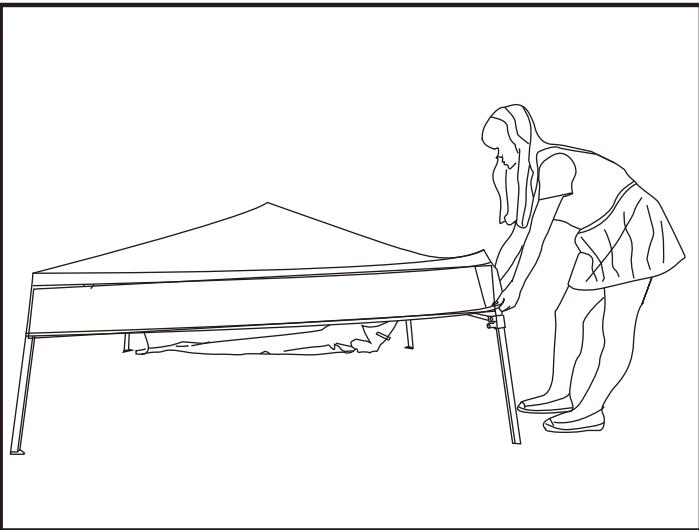
**EN** Place the canopy over the top frame. Use the Velcro pads to secure the canopy to the frame at each corner.
