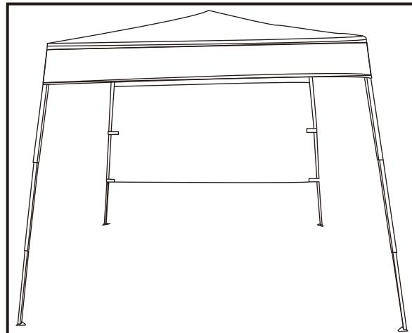
**EN** Drop the sunblock fabric wall and attach to the legs.
