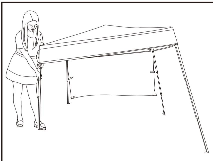
**EN** Gently pull out the telescoping legs stage by stage til the spring button pops in position. They are three stage telescoping legs. Please do not push in the spring button while pulling the legs and do not over pull each leg! You may lower the height by telescoping the legs back.
