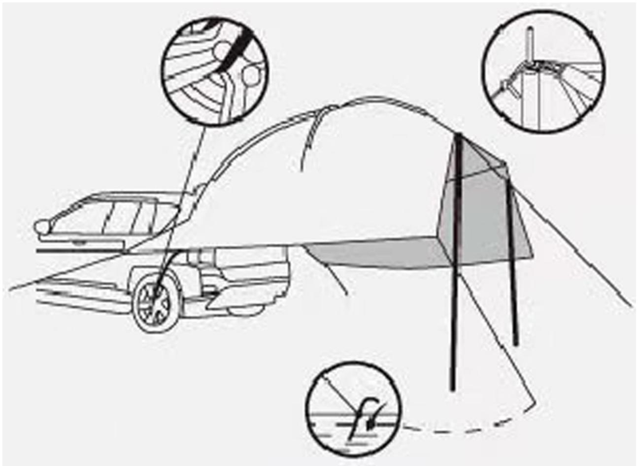
**EN\_2.** Tie the webbing at both ends of the tent to both sides of the rear wheels to fix it. Put the two poles on the other end of the tent and tighten it with a wind rope.
