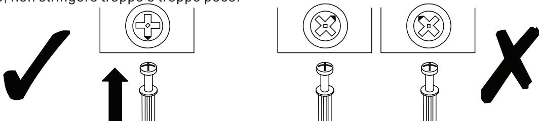
**EN\_CAM LOCK:** When fitting cam lock, ensure starting position is correct before you insert connecting quickfit.
