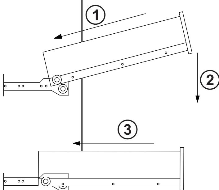
**EN** Be careful to push in the board when the both sides slide way been aligned.
