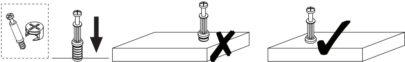
**EN\_QUICKFIT:** Tighten quickfit until shoulder is flush with panel. Do not overtighten or undertighten.
