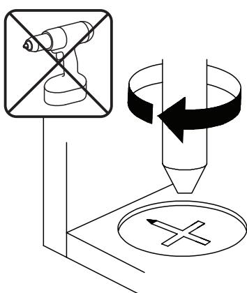
**EN**\_Turn cam lock clockwise to tighten.
