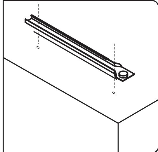
**EN** Please find the exact hole for installation, otherwise it will be misaligned. The screws on the drawer slide must be leveled , otherwise it will affect the smoothness of the d rawer.
