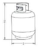
Max diameter: 300mm Max height: 430mm
