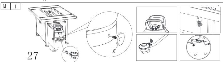
WARNING! Ensure the hose does not come into contact with any high temperature surfaces, or it may melt and leak causing a fire.
