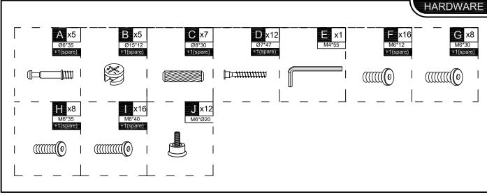
**EN\_**Do not confuse similar screws.Do not tighten bolts fully until all parts are connected!
